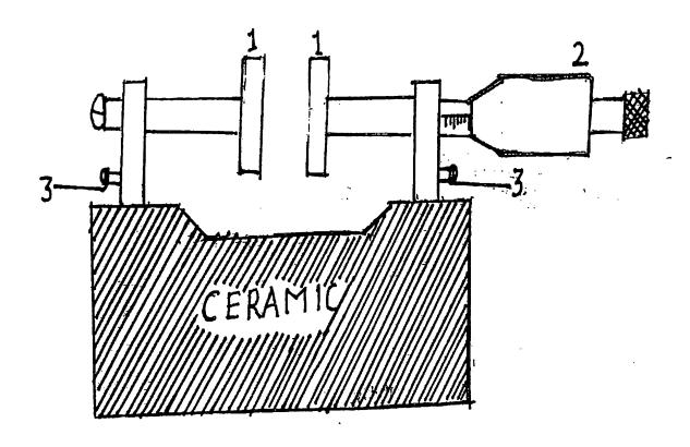
FIG.3: Schematic diagram of the sample holder for electrical conductivity measurements: 1, circular electrodes; 2, screw of a gauge; 3, measuring leads
